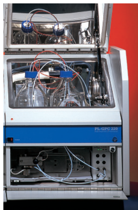
Figure 5. Agilent PL-GPC 220 integrated solvent delivery system
